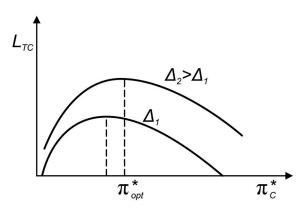
Fig. 2. Dependence of the work of the thermodynamic cycle  $(L_{TC})$  on the degree of pressure increase  $(\pi_{C}^{*})$  and the degree of heating of the working fluid  $(\Lambda)$
