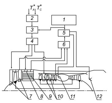
Fig. 3. Diagram of a hypothetical GTE for SST with a cold boost system.
