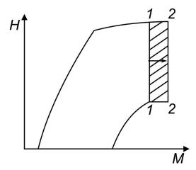
Fig. 4. The area of limitation of the operating modes of supersonic transport
